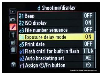
Mirror Lockup must be used with the timer. When you press the shutter button with mirror lockup set and timer set, the camera first pulls the mirror up. It then waits for the timer to trigger the shutter after the duration of the timer. This provides
