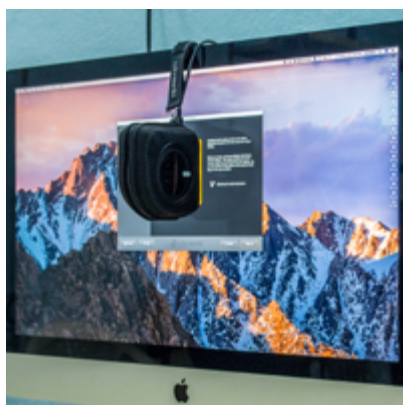
Picture 4: The colorimeter is attached to the face of the monitor and then the profiling software is run. This is how the setup will look when profiling is in progress.
