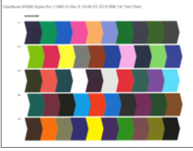
Picture 5: Reference color patches printed on the printer being profiled.
