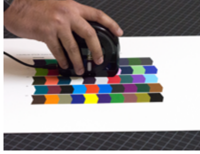
Picture 6: Color patches printed are read by the spectrophotometer to generate a profile for your printer.
