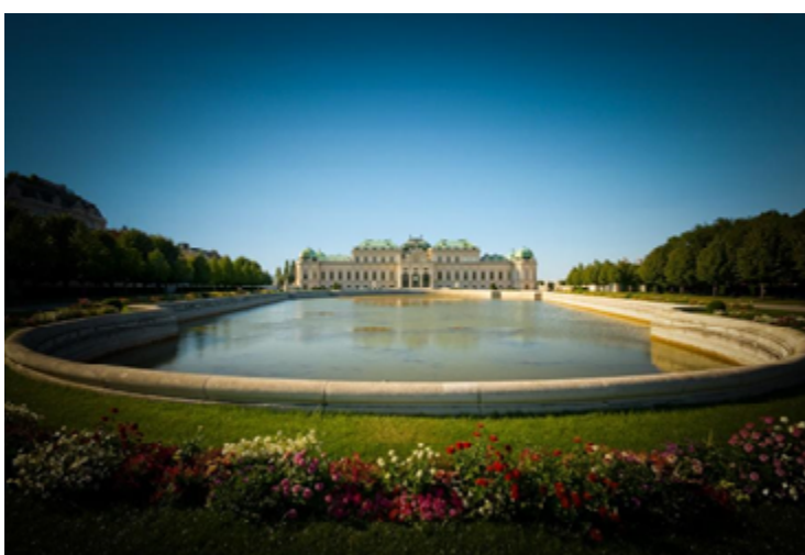
Picture 5: This is how the image will look if a lens designed for coverage of a cropped format is used on a full-frame camera. Note the heavy vignetting at the corners.
