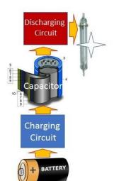
in simple terms, how a flash works. It uses a "Capacitor" to hold small currents at high voltages required to fire the Xenon flash lamp. The capacitor is charged to a high voltage by a charging circuit drawing power from the batteries we insert. It takes a few seconds to charge the capacitor making event photographers tense. When you click a picture, the discharging circuit is triggered and that sends power from the capacitor to the xenon lamp making the flash to fire.
